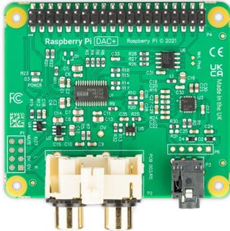
Raspberry Pi DAC+ is a high-performance audio HAT compatible with any Raspberry Pi computer that has a 40-pin GPIO header. With the Texas Instruments PCM5122, it delivers stereo analogue audio to a pair of phono (RCA) connectors. It does not require external power, and connects directly to Raspberry Pi's GPIO header with no need for soldering or cables.
