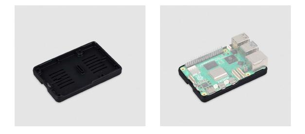
The Raspberry Pi Bumper for Raspberry Pi 5 is a snap-on silicone cover that protects the bottom and edges of the board.
