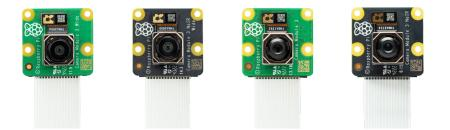
Raspberry Pi Camera Module 3 is a compact camera from Raspberry Pi. It offers an IMX70812-megapixel sensor with HDR, and features phase detection autofocus. Camera Module 3 is available in standard and wide-angle variants, both of which are available with or without an infrared cut filter.
