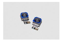
The Raspberry Pi Camera Module 3 Sensor Assembly contains the same sensor and autofocus functionalities as Raspberry Pi Camera Module 3 AF (autofocus), enabling you to integrate the features of Camera Module 3 into a more diverse range of form factors. This assembly provides a low-cost way to add imaging capability to smaller devices, reducing manufacturing complexity and time to market.
