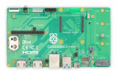
The Raspberry Pi Compute Module 5 IO Board provides a starting point for those wishing to integrate Raspberry Pi Compute Module 5 into products, while also serving as an alternative Raspberry Pi form factor for industrial applications.
