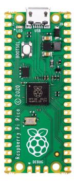
Raspberry Pi Pico is the debut microcontroller-class board from Raspberry Pi. Built around our RP2040 silicon platform, Pico brings our signature values of high performance, low cost, and ease of use to the microcontroller space.
