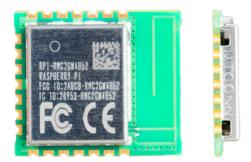
Raspberry Pi Radio Module 2 is a radio module designed for use with Raspberry Pi's low-cost, high-performance microcontrollers. It uses Infineon's CYW43439, a single-chip combo device featuring 1×1 single-band 2.4GHz Wi-Fi<sup>®</sup> 4 (802.11n) and Bluetooth<sup>®</sup> 5.2 for low-cost applications. It is a small form-factor solution with minimal external components for reduced mass production costs.
