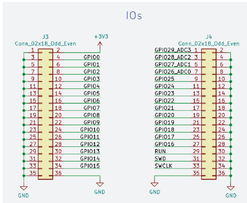
Figure 10. Schematic section showing the 2.54mm I/O headers
