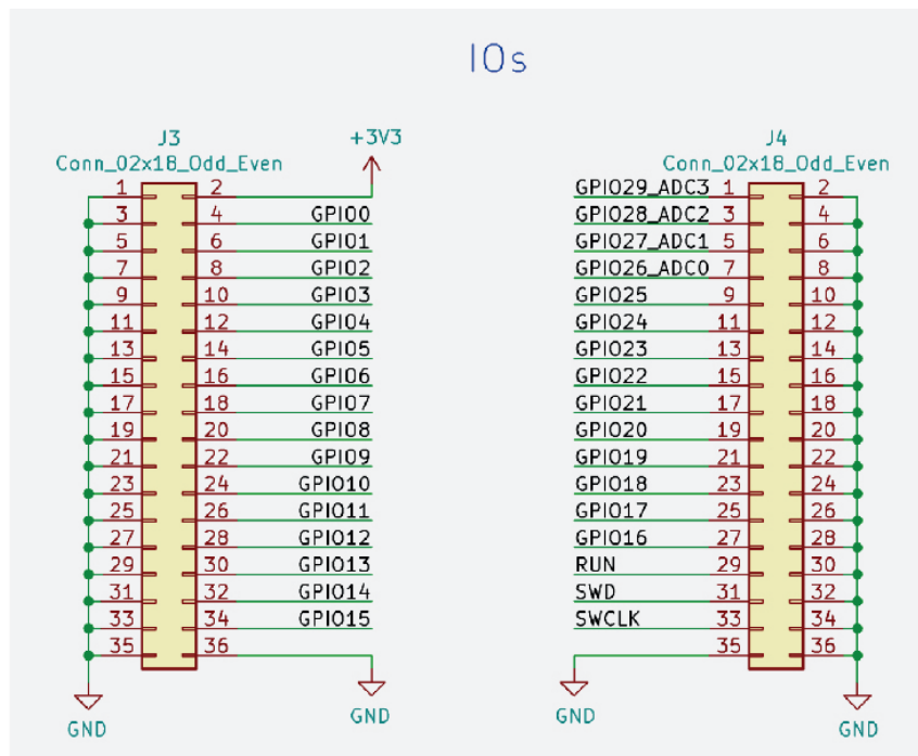
Figure 10. Schematic section showing the 2.54mm I/O headers
