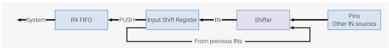
Figure 46. Input Shift Register (ISR). Data enters 1...32 bits at a time, and current contents is shifted left or right to make room. Once full, contents is written to the RX FIFO.
